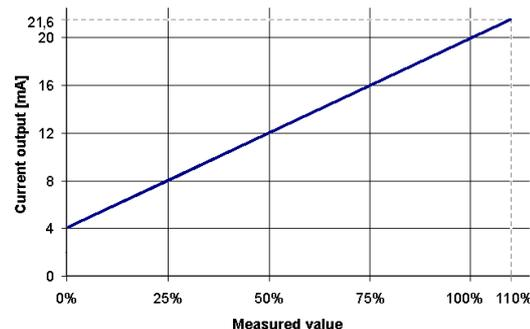
Fig 34 Current output 4-20 mA (Standard)
