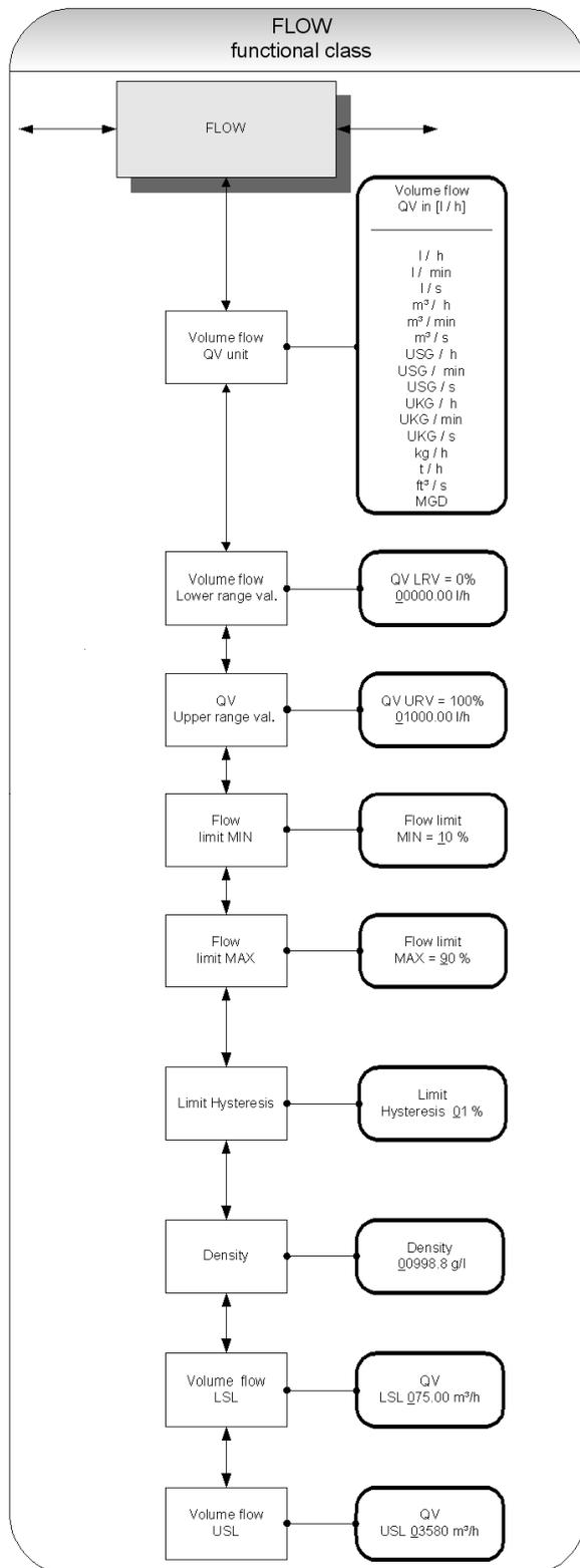
Fig 27 Functional class FLOW incl. all submenu items
