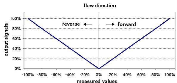
Fig 41 Output signals (setting **forward & reverse**)
