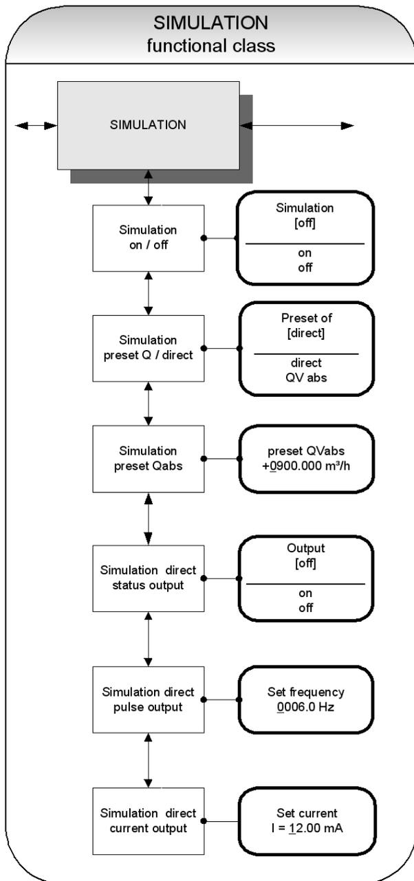
Fig 36 Functional class SIMULATION incl. all submenu items
