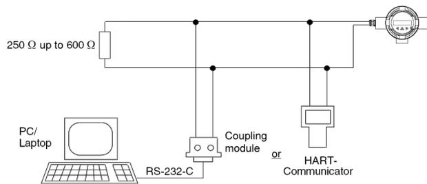
Fig 16 Electrical connection for HART® communication, schematic diagram
