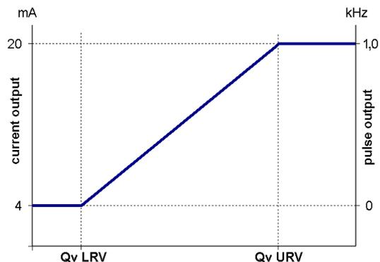
Fig 28 Output scaling of the mag-flux M1
