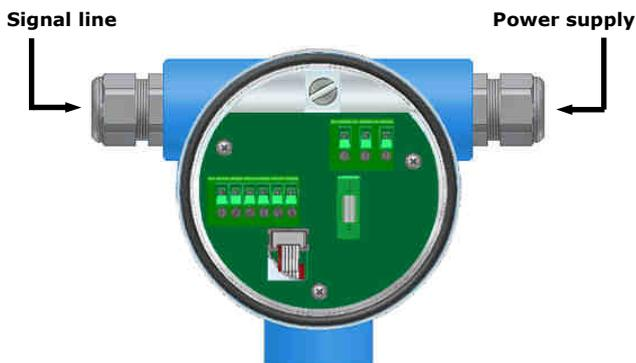
Fig 8 Electrical connections of the transmitter *mag-flux M1*
