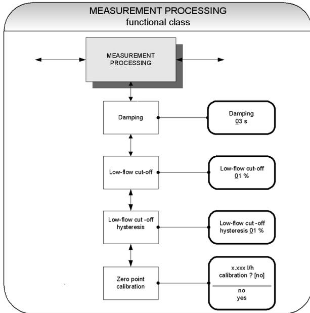
Fig 26 Functional class MEASUREMENT PROCESSING incl. all submenu-items
