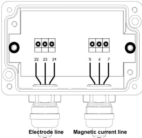
Fig 11 Connection diagram for sensor cable of the *mag-flux M1*
