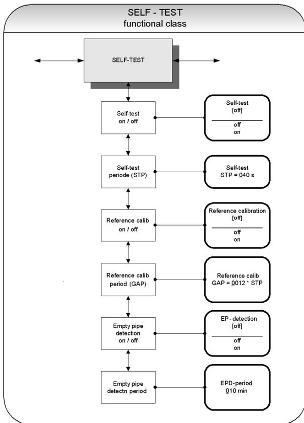
Fig 37 Functional class SELF-TEST incl. all submenu items
