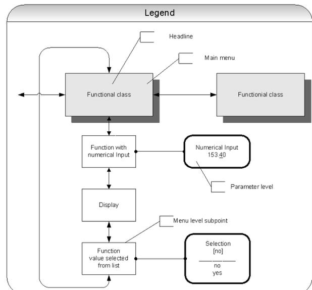
Fig 21 Structure of the mag-flux M1 user interface
