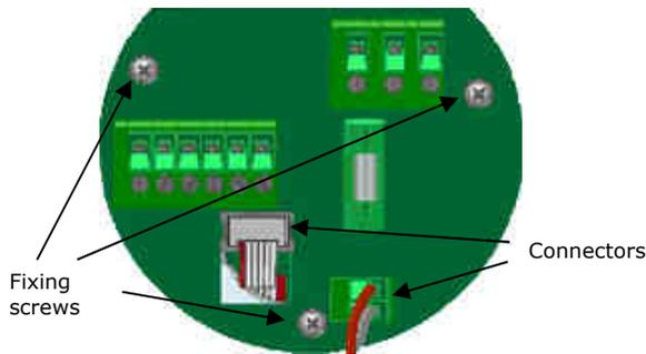
Fig 18 Terminal board of the *mag-flux M1*
