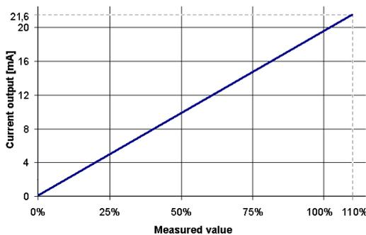
Fig 33 Current output 0 - 20 mA
