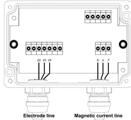
Fig 12 Electrical connections of the *mag-flux A* sensor
