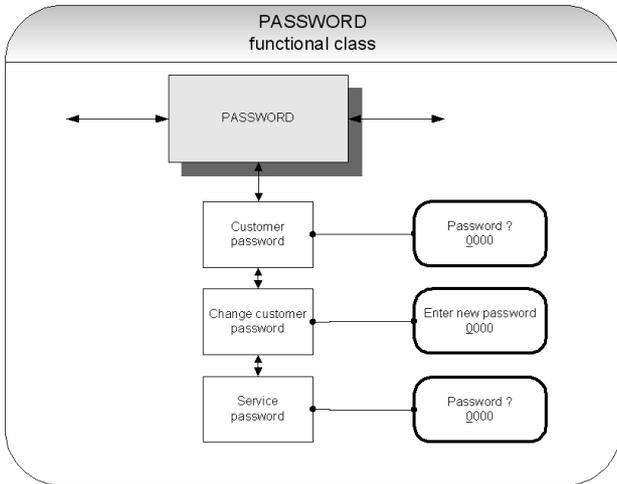
Fig 24 Functional class PASSWORD incl. all submenu items
