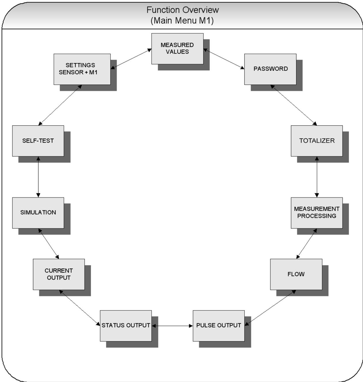
Fig 22 Main menu *mag-flux M1* (functional classes)
