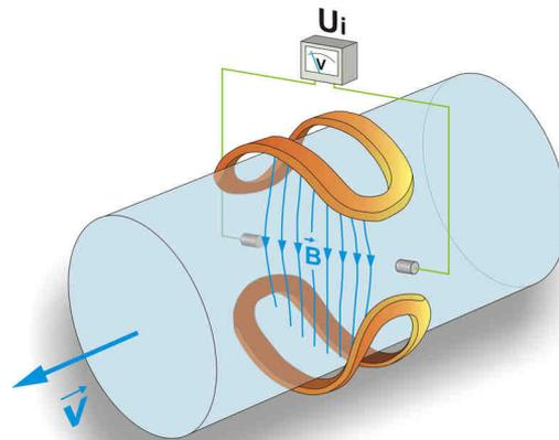
Fig 2 Principle of the magnetic-inductive flow measurement
