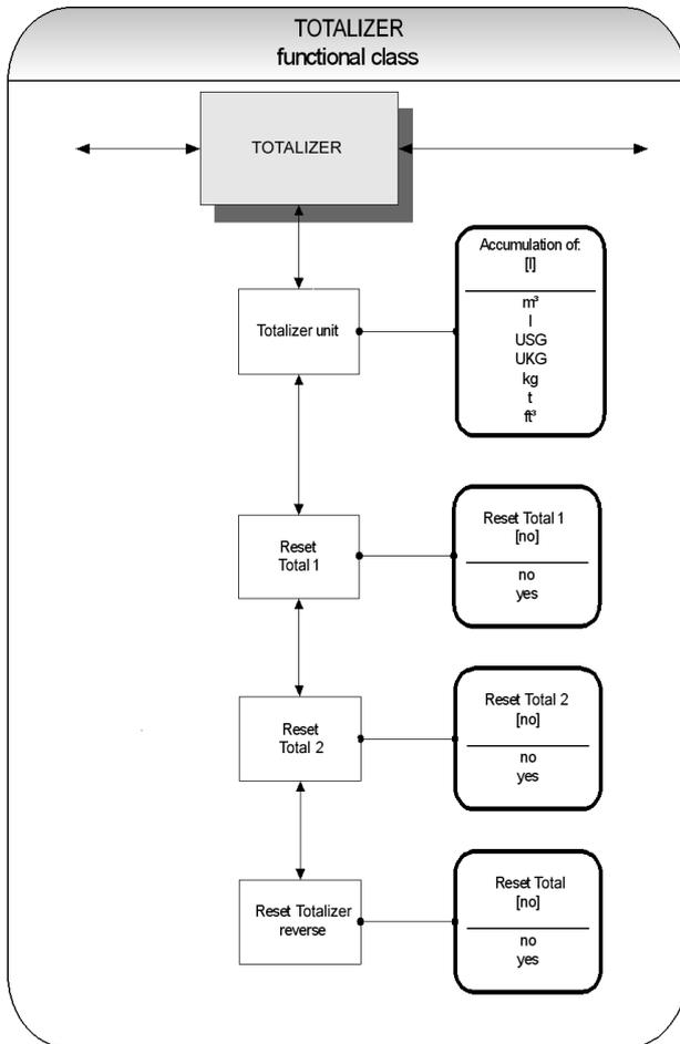
Fig 25 Functional class TOTALIZER incl. all submenu items
