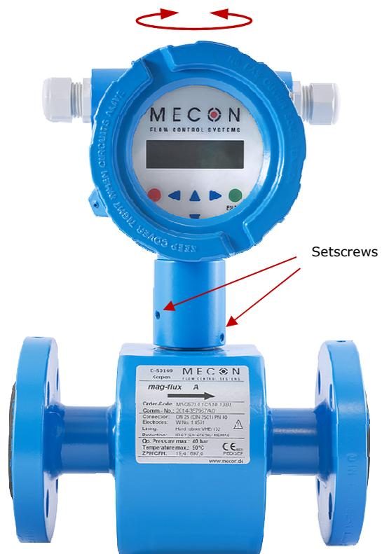
Fig 17 Position of the setscrews for changing the orientation of the transmitter housing (*mag-flux A compact*)
