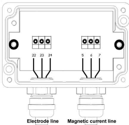
Fig 9 Electrical connection of the *mag-flux M1*
