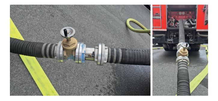
The suction simulation trainer (AST) is designed for use in the suction lines of fire pumps. The AST realistically simulates different operational situations in suction operation, such as the water column breaking off, cavitation or failure of water delivery due to blockage of the suction strainer, falling water level in the water supply point or leaks in the suction line.
